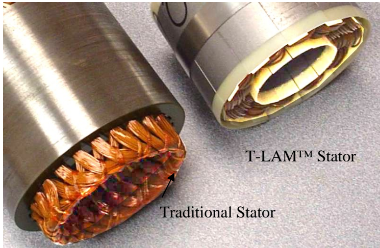
Figure 4: End turn length comparison
