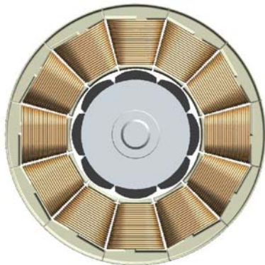
Figure 3: Minimized, non-overlapping end turns
