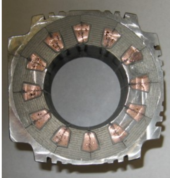
Figure 11 – Cross-Section of Potted T-LAM Stator
